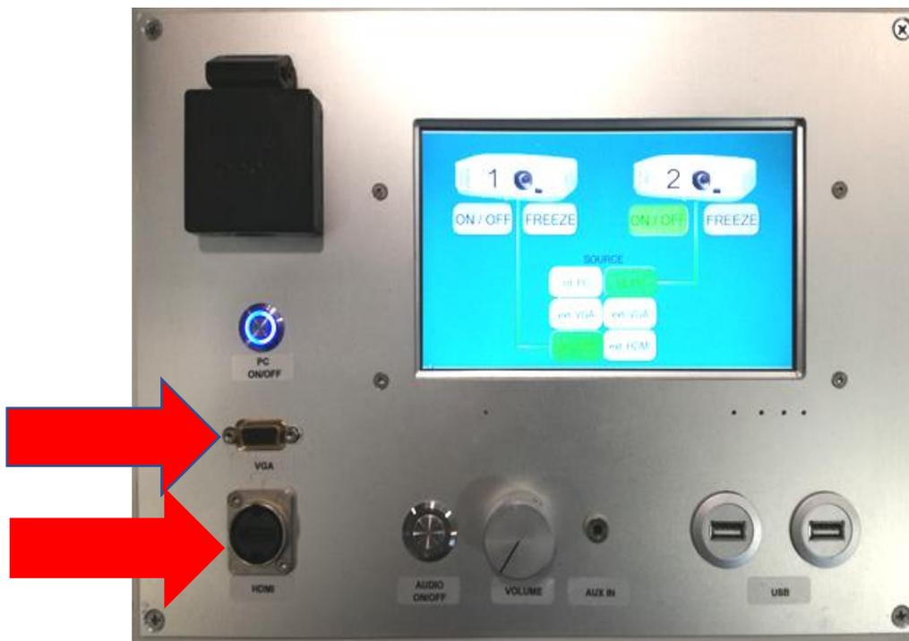
With the "ON/OFF" button on the control panel you can switch the desired projector on or off
