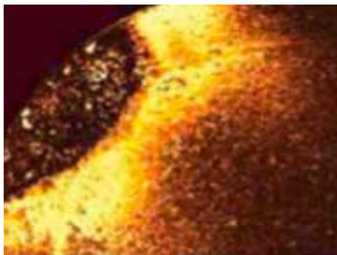
Element map for iron on an indexable insert of cubic boron nitride
